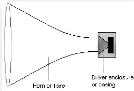
*The horn transforms high pressure and low velocity movement from the speaker driver at the horn throat to low pressure and high velocity at the horn mouth by impedance matching.*
