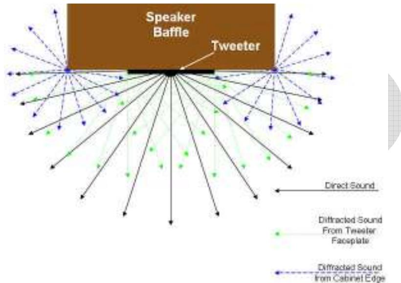
*Edge diffraction messes up the speakers polar response, making it look like the back of a porcupine.*
