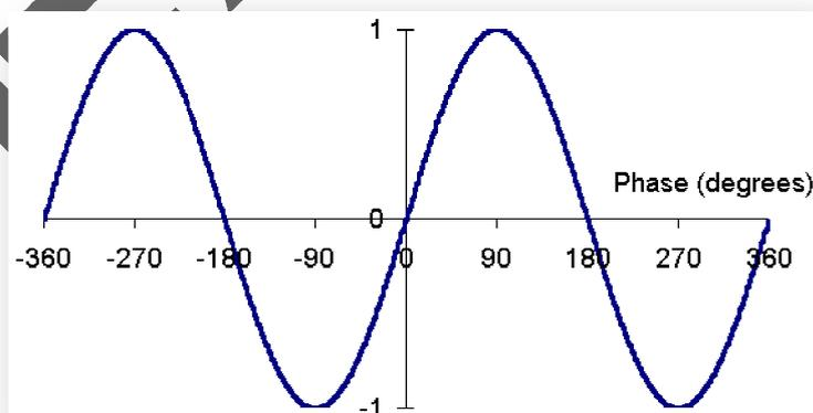
*Picture shows a sinewave over two full cycles. The X axis shows the angular relationship but could also be time as frequency =1/t. The Y axis is the level or amplitude.*
