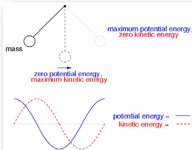
*A swinging pendulum translates potential energy into kinetic energy over its cycle. The swinging action can be projected into a sine curve revealing the 90 degree phase-shift in between the two states. This relationship is everywhere in nature and in science, understanding it, is very useful. The picture shows a simple harmonic motion, the basic oscillation.*
