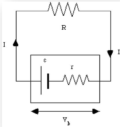
If you apply OHM's law here where P is voltage multiplied by current, you will find that when the battery is loaded (R in the picture) by something with a resistance equaling the battery Ri, maximum power is produced. Note POWER, not current and not voltage, but the product of the two is at its peak when source and destination R's are equal matches.
