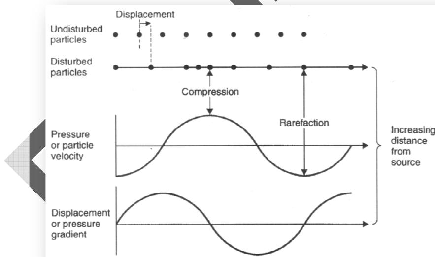
*In the two pictures above and below (courtesy John Watkinson, "The art of sound reproduction") we may see the relationship between pressure and velocity of sound. Also seen is how the slope is a function of frequency and amplitude and why larger drivers are required for lower frequencies*
