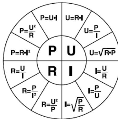
*P stands for power, U for voltage, R for resistance and I for current. This electrical model has many analogies in other disciplines giving an intuitive sense for physics.*
