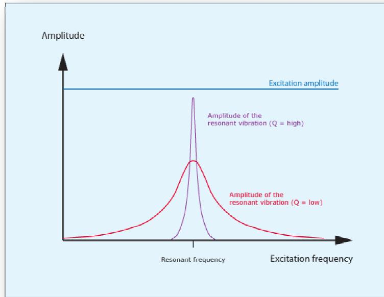
*Q is a dimensionless factor in resonance where a high Q means the peak is high and bandwidth small. Even though incorrect use, Q is used for instance to describe the type of roll-off in a reflex speaker. Often the designer chooses the Q such that a pronounced gain occurs just before response rolls of. This accounts for the false impression of low bass found in such designs*
